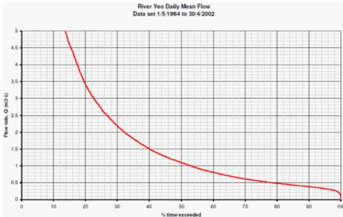
Figure 1 – Long-term flow duration curve for the River Yeo in Somerset.
